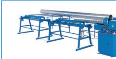
Standard Run-off Table duct length up to 3m, including automatic discharge
