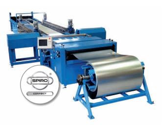
>> Unique modular approach to boost your Spiro® Ductline into a fully automatic rectangular duct forming line with integrated flanges – expand gradually or at once, you decide.
